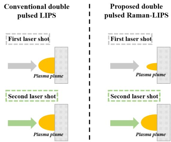
[Fig.1] A schematic of double pulsed Raman-LIPS system
