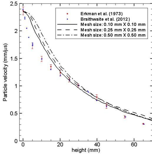
Fig. 3 Mesh refinement test via particle velocity.
