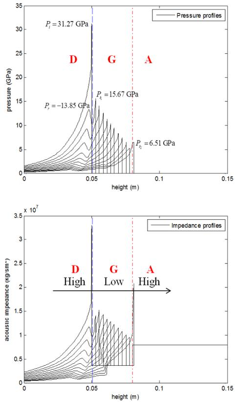
Fig. 9 Pressure and acoustic impedance of LSGT simulation (Donor, Gap, Acceptor).
